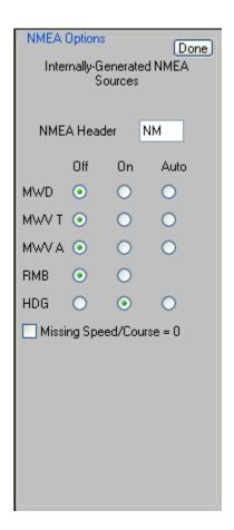
NavMonPc provides several "generated" NMEA outputs, as described in the user's guide. This revision adds HDG, which sends the magnetic HDG as displayed on the NavMonPc dials. HDG also sends the magnetic variation as used by NavMonPc.
