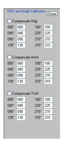
There is now the ability to scale, and in some cases offset many of the data decoded by NavMonPc. Two windows contain the calibration options. The calibration factors entered here are applied to the data inputs. The corrected values are shown on the NavMonPc displays, and are used by the NMEA generators. The original NMEA sentences received by NavMonPc are not modified, and are sent out the output ports as-is.
